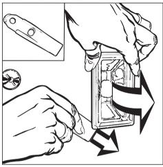
■ Change the halogen lamp: 12 V, 20 W, heat resistant to 300°C, Osram, Type w969.
